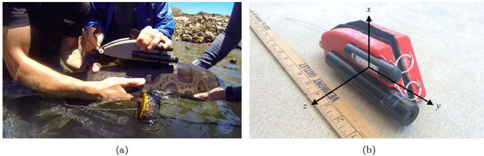
Figure 5. An image of the tag on a leopard shark fin (a). The coordinate axis used for the magnetometer readings (b).
